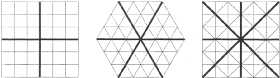
Figure 7.5 Directions of strut proliferation for bi-, tri- and quadri-directional tensegrity grids
